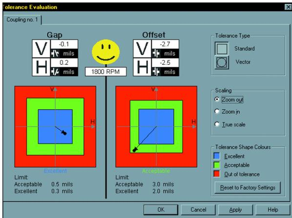
**Figure 5. Results of using standard tolerances**
