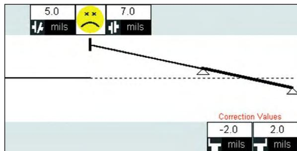
**Figure 8.** Small correction values at the feet do not necessarily reflect good alignment at the coupling.
