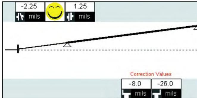
**Figure 9. Using improperly specified tolerance values at the feet**
