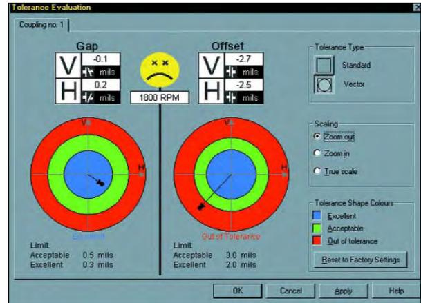
**Figure 6. Results of using vector tolerances**
