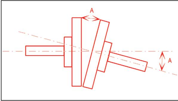
**Figure 4. Measuring the angle between shaft centerlines**
