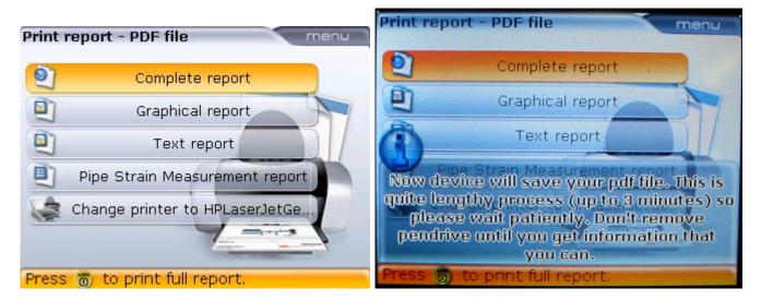
You may have to wait as long as three minutes before the report has been generated and saved on the memory stick. Do not remove the stick or press any buttons you get the following screen:
