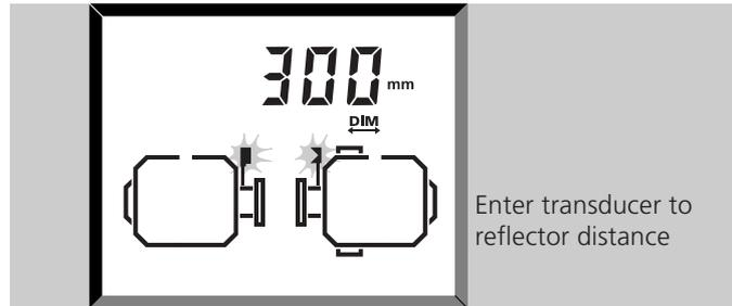
Measure from the marking on top of the transducer housing to the marking on top of the reflector.
