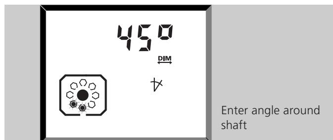
Enter the angular position around the flange of the bolt. The angle is defined clockwise in degrees, starting with  $0^\circ$  corresponding to the 12 o'clock position as defined on page 5-6.
