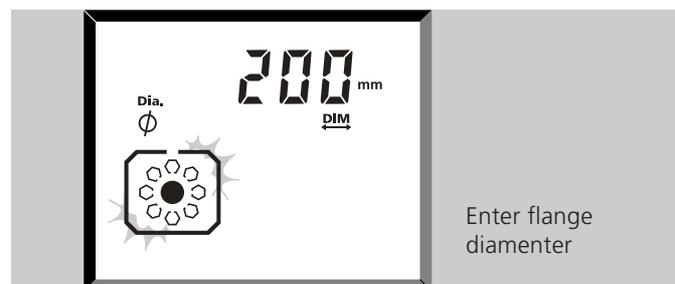
Enter the outer diameter of the flange. This is the point where the upper machine rests and tilts on the lower machine. It is used to calculate the minimum number of shims at each bolt to separate the flange. The bigger the flange, the more shims required.
