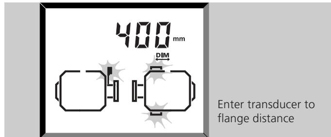
Enter the distance between the marking on the top of the transducer and the center surface of the flange.
