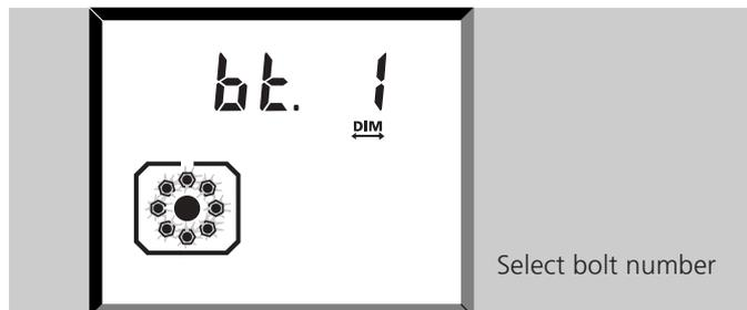
We now define the positions of the flange bolts in order to calculate their shimming requirements..
