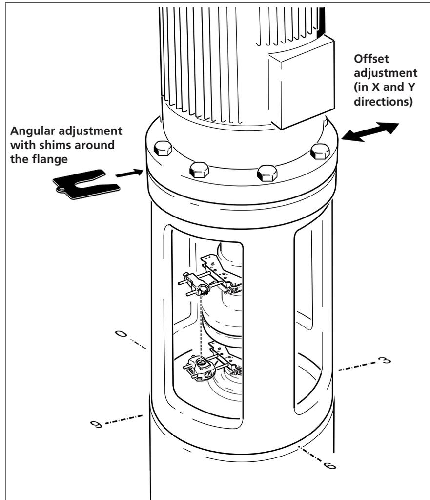
The OPTALIGN PLUS transducer and reflector are mounted on either side of the coupling as for horizontal machines, with the transducer below and the reflector above. Measurements are then made at a series of 90° or 45° rotational positions.
