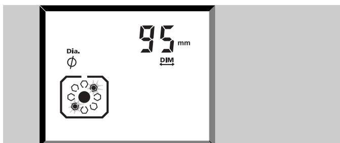
Type-in the *diameter* at which the bolt lies. This is TWICE the distance from the shaft center to the bolt.
